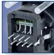
Vertical PCB with lightpipes
