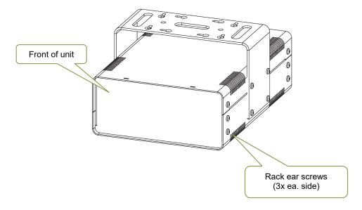
3) The drawing below depicts the 2U Large Single (top) and Dual (bottom) RackMount Kits. Note the Dual version requires TWO center Dual Joiners (included in the Kit), attached at the front and rear of the units, enhancing stability in the rack. The same principle applies to Small Dual (for IQ and Opto Mini enclosures), and Medium Dual (for GBS Mini) RackMount Kits.
