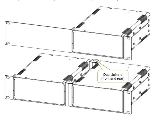
4) Caution: Mounting ProPlex FloppyDrives, Mozart Drives and IMS Universe Drives. These LED driver units must have adequate airflow. When installing multiple units, they must be mounted on alternating sides of the rack, so one does NOT reside directly above another, with at least one-half 1U space between each assembly, per below illustration. Other ProPlex PortableMount units – IQ, GBS, Opto-Splitter, etc. – may be mounted adjacent to each other.
