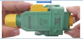
Slide the unlocking protection over the housing from the cable side to prevent unintentional unlocking.
