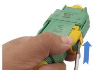
To open the connector / remove the release protection, insert a screwdriver (e.g. flat-bladed | 0.8 x 4 mm) into the opening provided in the protective cover (see fig.) and press the release spring inside upwards.
