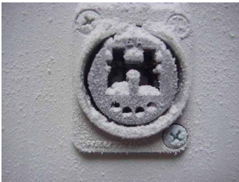
figure 10.c: Dust sediment on the front side of the receptacle after 60 min.
