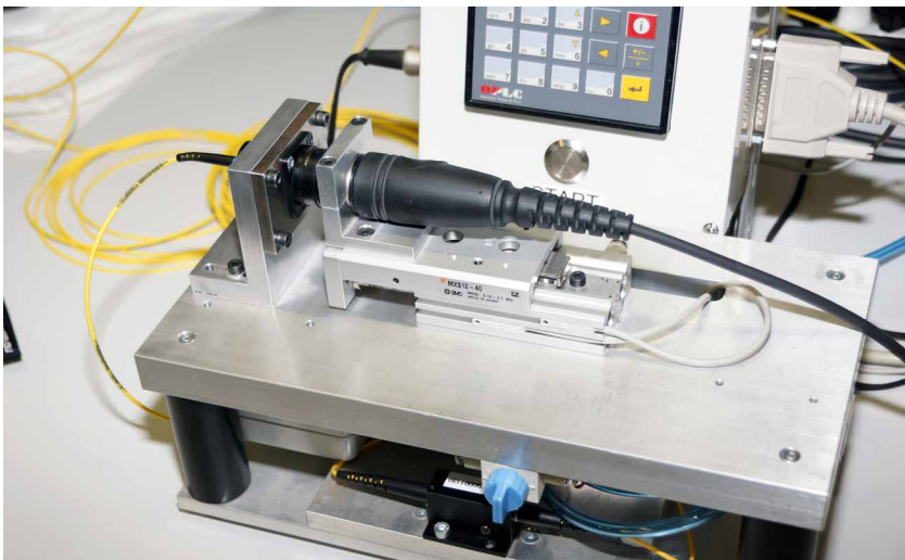
figure 6.b: fixture for 500 and 5.000 mating cycles
