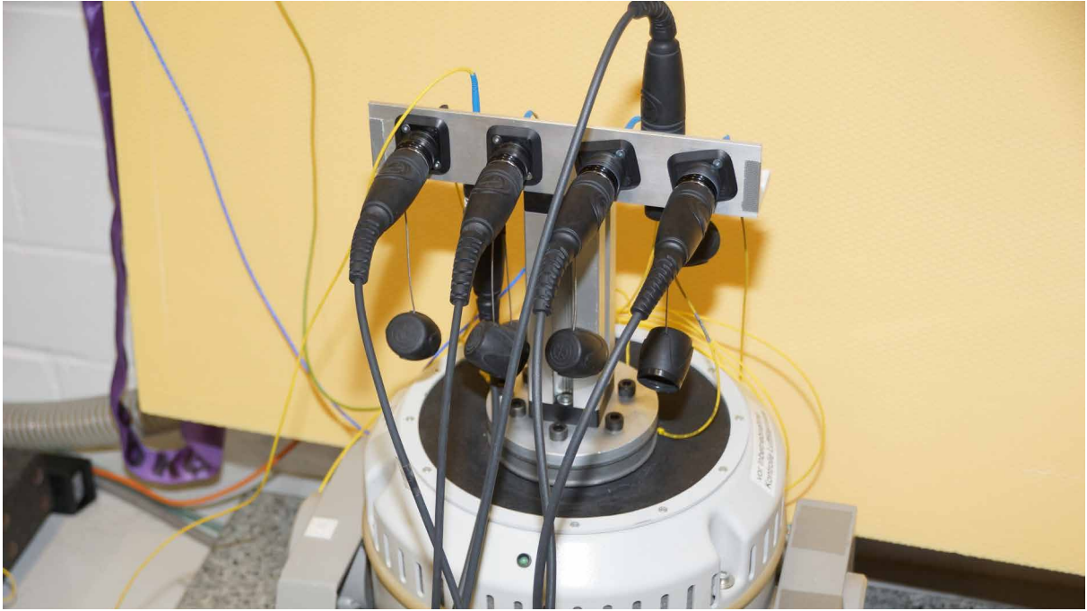
figure 2.a: Vibration equipment and test cable arrangement
