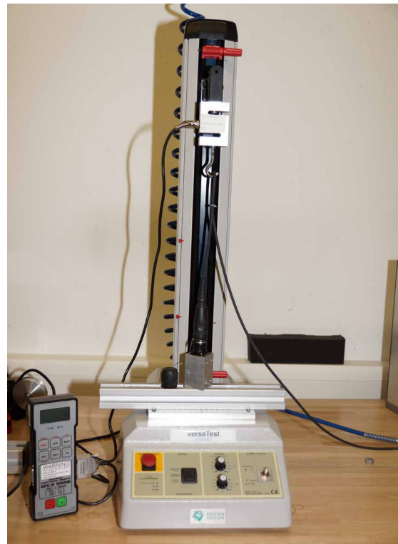
figure 3.a: Equipment for examination of cable retention
