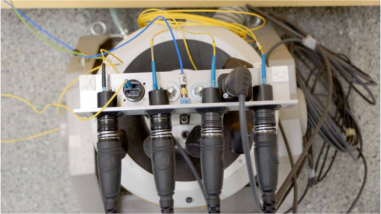
figure 2.b: : Vibration equipment and test cable arrangement
