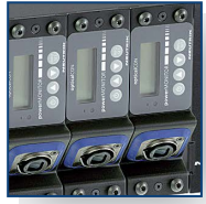
3RU frame with up to 9 powerMONITORs
