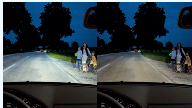
Left: Light distribution with XENARC® lights – Right: Light distribution with halogen lights
