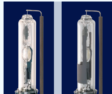
S-type: The cut-off line is created by a shield (left). R-type: To generate the cut-off line in the light distribution a black coating is applied directly on the outer bulb of the lamp (right).
